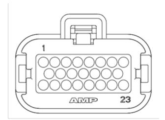
The connector and terminals models related to vehicle wiring harness: AMP 770520-1/770854-1; AMP 770680-1 (plastic housing)
